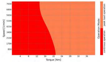
Note: Assuming water temperature of 40°C and 7 l/min flow.
