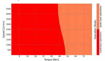
Note: Assuming water temperature of 40  $^{\circ}\text{C}$  and 7 l/min flow.
