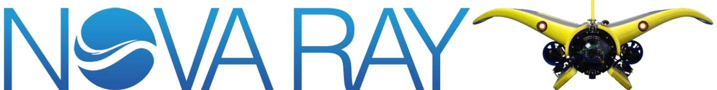
The Nova Ray's unique hydrodynamic features effectively use water flow rather than resistance to maintain operational control under changing operating modes. Under thruster power, the wings operate just as a high-winged airplane would in free flight. Under "controlled" tow, the arcuate wing, combined with the seamless shift in the center of rotation from the cable pull, produces a stable configuration through the water column.
